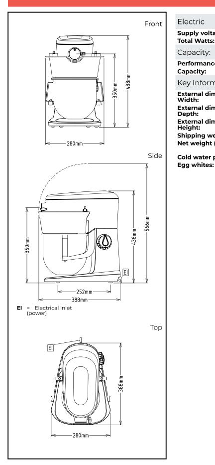
Electric Supply voltage: 200-240 V/1N ph/50/60 Hz **Total Watts:** 0.5 kW Capacity: Performance (up to): 0.75 kg/Cycle Capacity: 5.5 litres Key Information: External dimensions, Width: 280 mm External dimensions, 388 mm Depth: External dimensions, Height: 438 mm 15.6 kg **Shipping weight:** Net weight (kg): ISO 9001; ISO 14001 0.75 kg with Semi spiral **Cold water paste:** hook
